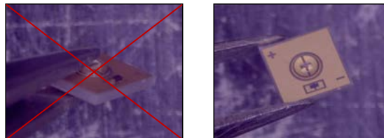
Fig 10. incorrect handling (left) and correct handling (right) of UVC LED Package
